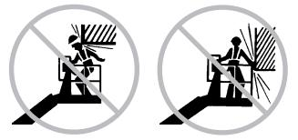
Be aware of crushing hazards when grasping the platform guard rail.
