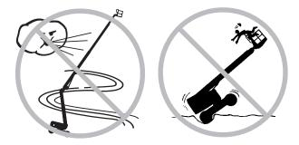
Use extreme care and slow speeds while driving the machine in the stowed position across uneven terrain, debris, unstable or slippery surfaces and near holes and drop-offs.
