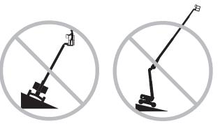
Do not depend on the tilt alarm as a level indicator. The tilt alarm sounds in the platform only when the machine is on a severe slope.
